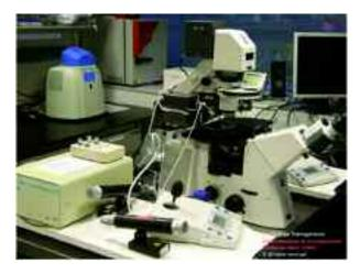
Zeiss AxioObserver-D1optical inverted microscope and motorized micromanipulators used for the production of genetically-modified mice.
